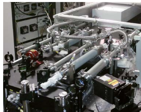
12 J @ 527 nm laser system during development stage
