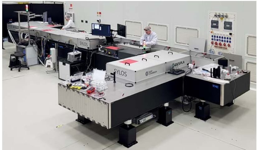
Fig 7. Typical external view of APL1301k-x4-SH laser system pumping OPCPA (ELI-ALPS, SYLOS2A system)
