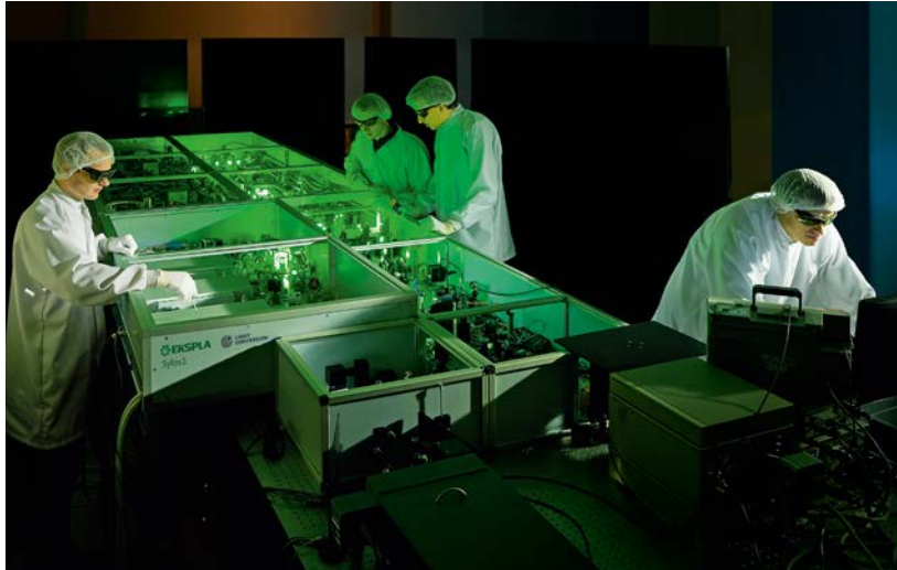
Unique OPCPA based laser system, providing ~5 terawatts of output power at 1 kHz repetition rate has been designed and built for ELI-ALPS facilities located in Szeged, Hungary
