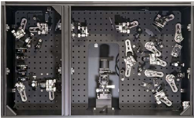
Spectroscopy module of Phase-sensitive SFG spectrometer: internal view (left) and 3D drawing (right).
