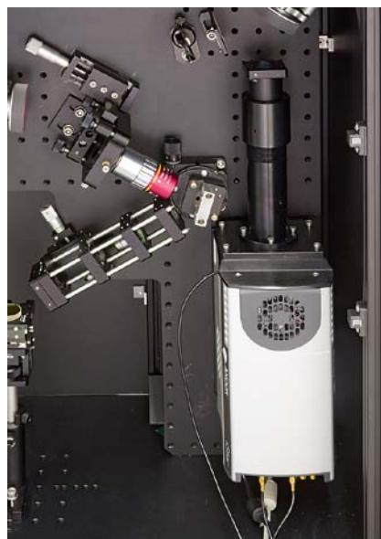
Detection part of SFG microscope.
