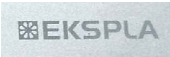
Fig. 1. Digital camera (left) and optical microscope (right) images of Ekspla logo marked on silicon wafer. The marking resolution was 50 μm in both transverse x and y directions.
