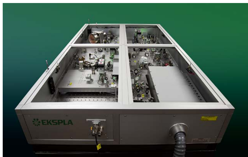
UltraFlux FT2105HE. Customised compact (1.2 × 0.9 m), fully diode pumped, tunable wavelength femtosecond laser system delivering up to 2.5 mJ pulse energy with pulse duration down to 20 fs. Optically synchronized (low jitter) fs and ps outputs available.
