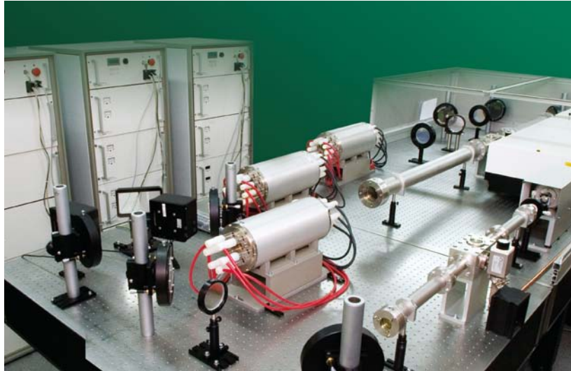
160 J @ 1053 nm MM laser system
