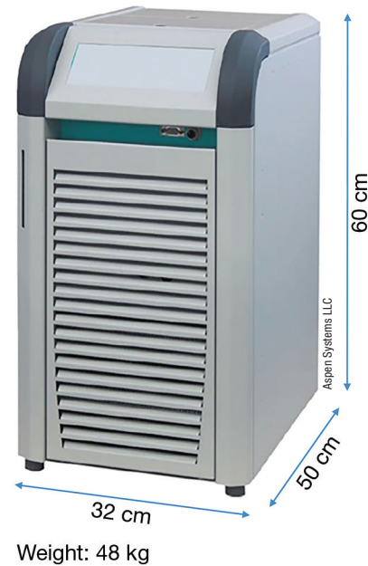
Figure 1. Left: A typical pumped-loop liquid chiller. These systems use single-speed compressors paired with large reservoirs to stabilize coolant temperatures during load fluctuations and compressor cycling.
