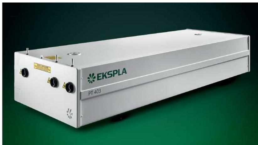
PT403 series laser systems integrate a picosecond 1 kHz repetition rate DPSS pump laser and optical parametric generator into a single housing. New picosecond tunable wavelength laser system provide from 210 to 2300 nm from the one box.
