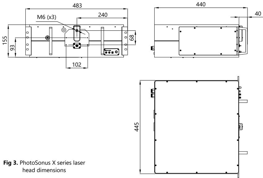
**Fig 3.** PhotoSonus X series laser head dimensions
