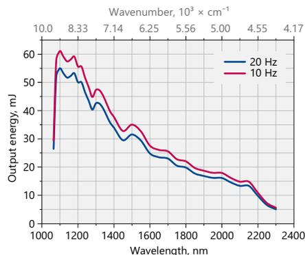
**Fig 2.** Typical PhotoSonus M-10 and M-20 Idler output pulse energy vs. wavelength curve
