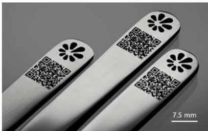
Black marking of tweezers. Courtesy of FTMC.
