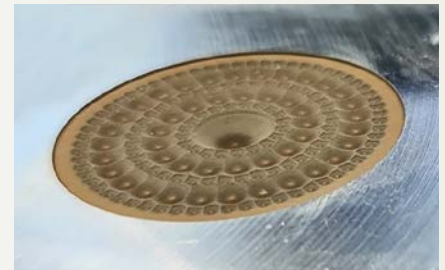
Textured aluminum molds. Courtesy of FTMC.
