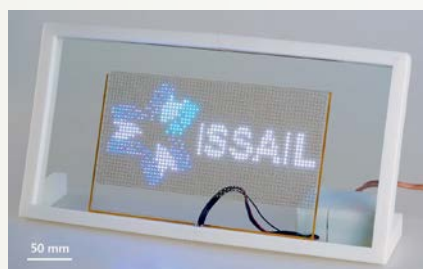
SSAIL technology on PA4T. Courtesy of Akoneer.
