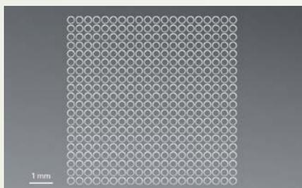
300 μm hole drilling in thin borosilicate glass.
