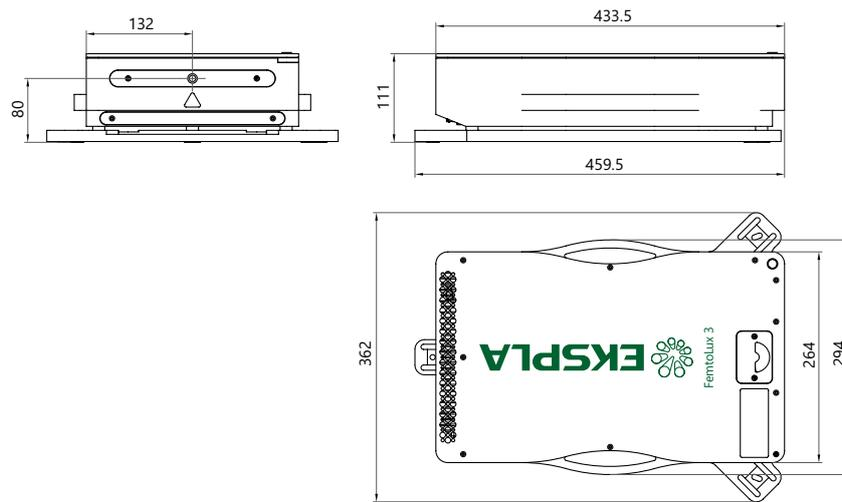
**Fig 10.** Outline drawings of FemtoLux 3 laser head
