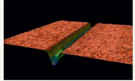
Optical 3D profilometer image of formed groove.
