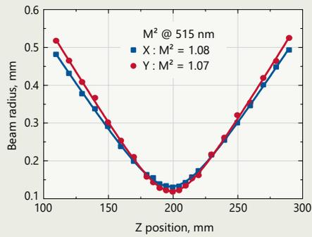
**Fig 7.** Typical M<sup>2</sup> measurement of FemtoLux 3 at 1030 nm (left) and 515 nm (right)
