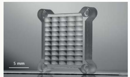
Cutting custom micro-lens array substrate from thick fused-silica glass.
