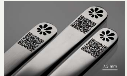
Black marking of tweezers. Courtesy of FTMC.
