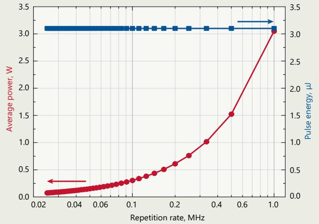
**Fig 4.** Typical dependence of output power and pulse energy of FemtoLux 3 laser at 1030 nm when repetition rate is reduced by pulse picker. Internal repetition rate of the laser in this case is 1 MHz
