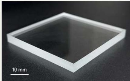
Laser-based Bessel beam scribing of 4.8 mm soda-lime glass.
