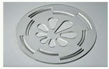
Fused-silica milling. Courtesy of FTMC.
