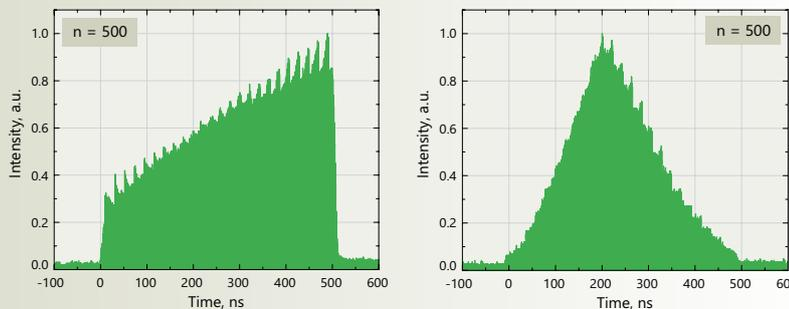
**Fig 5.** Measured 2.2 GHz pre-shaped bursts of 500 pulses at 233 kHz burst repetition rate for the desired rising burst shape
