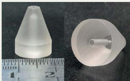
Glass nozzle fabrication by using multi-step bottom-up milling.
