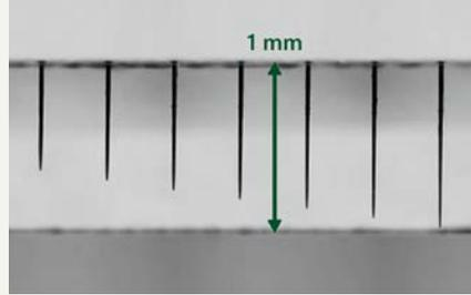
GHz burst assisted percussion drilling of high aspect ratio holes in EXG glass.
