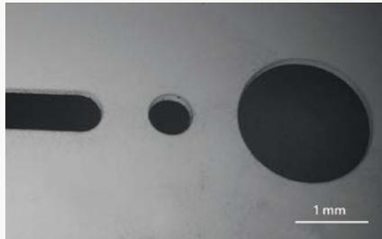
125 µm thickness tantalum cutting.
