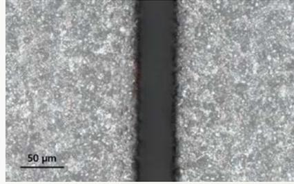
50 µm depth groove formation in ceramic.
