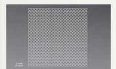
$300~\mu m$  hole drilling in thin borosilicate glass. Courtesy of FTMC.
