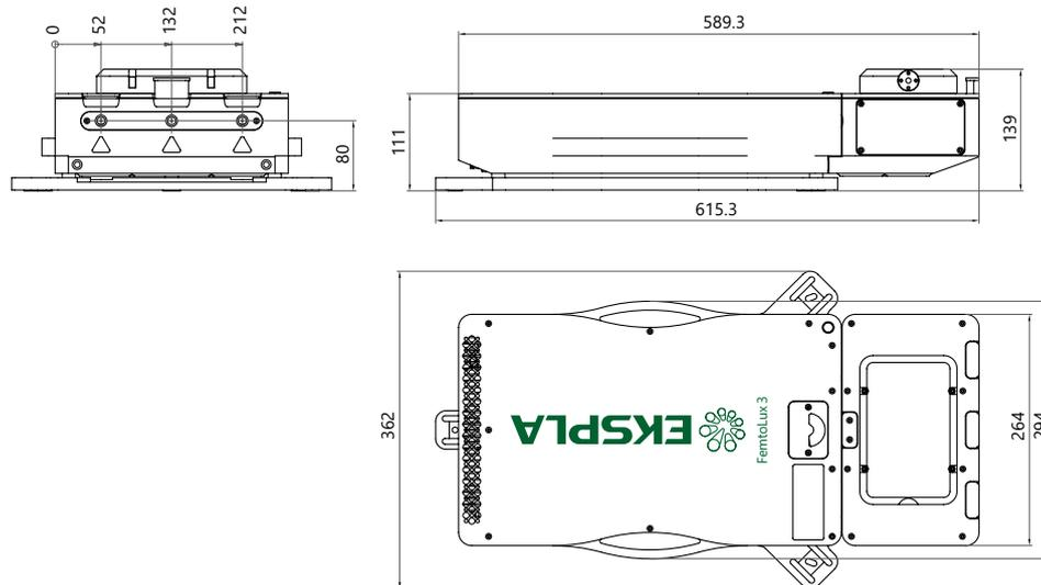
**Fig 11.** Outline drawings of FemtoLux 3 laser head with second harmonic option
