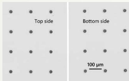
Bottom-up milling of 100 μm diameter taper-free channels in glass.
