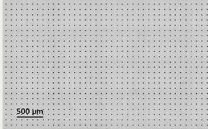
GHz burst assisted percussion drilling of high aspect ratio holes in EXG glass.
