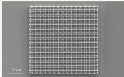
SEM image of photopolymerization sample.
