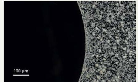
SEM image of processed FZ-Si wafer edge.
