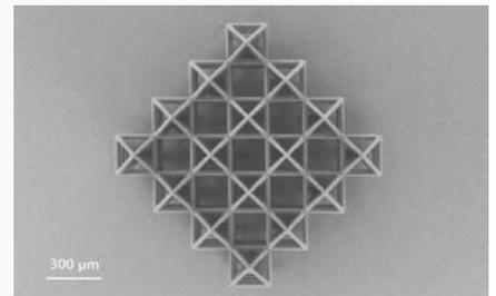
SEM image of photopolymerization sample.
