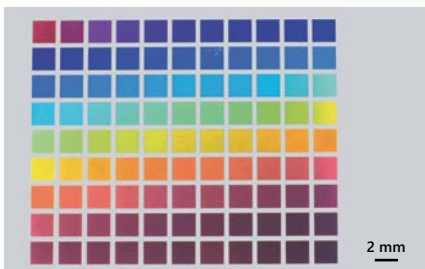
Titanium film coloring with GHz burst feature. Courtesy of Akoneer.
