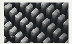
Bottom-up milling of fused-silica glass. Courtesy of FTMC.
