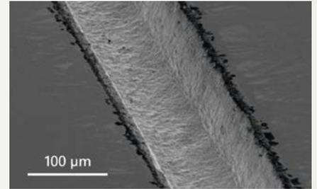
Groove formation in GaAs in water environment.
