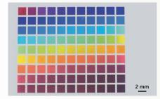
Titanium film coloring with GHz burst feature. Courtesy of Akoneer.
