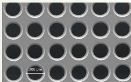
SEM image of 300 μm holes in borosilicate glass.
