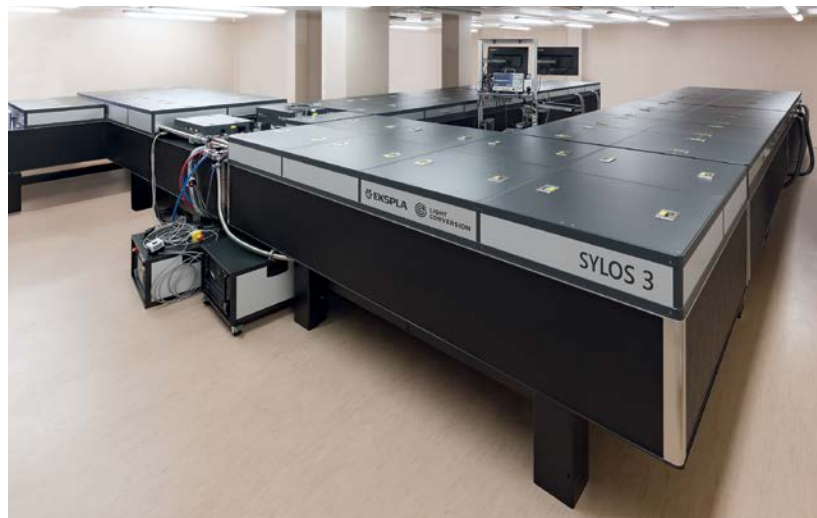
Unique OPCPA based laser system, providing ~15 terawatts of output power at 1 kHz repetition rate and an 8 fs pulse duration. Has been designed and built for ELI-ALPS facilities located in Szeged, Hungary
