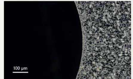
SEM image of processed FZ-Si wafer edge.
