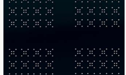
Selective laser etching (SLE) of through-glass vias in glass. Courtesy of WoP.
