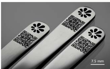
Black marking of tweezers. Courtesy of FTMC.
