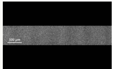
Scribed 1 mm soda-lime side wall view. Courtesy of FTMC.
