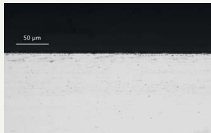
Scribed 4.8 mm soda-lime edge view. Courtesy of FTMC.
