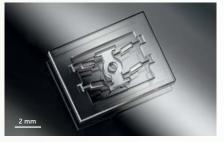
Femtosecond laser induced selective etching of bistable switch.
