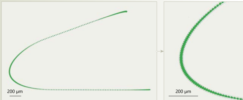
Fig 1. Complex shape scanned with time based laser triggering mode with a pulse repetition of 200 kHz and scanning speed of 6 m/s. The scanning started from the top right to the bottom right area. Overlapping pulses result in an overheated area.
