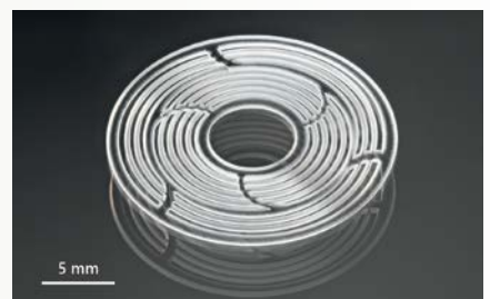
Thin fused-silica cutting. Courtesy of FTMC.
