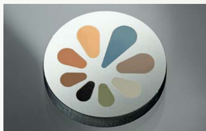
Color marking of stainless steel. Courtesy of Akoneer.
