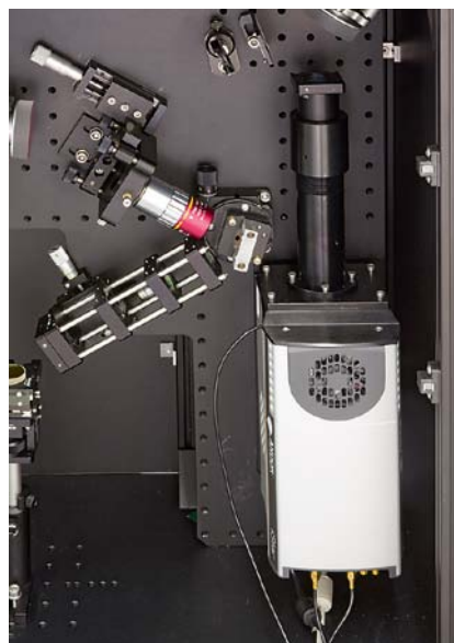
Detection part of SFG microscope.
