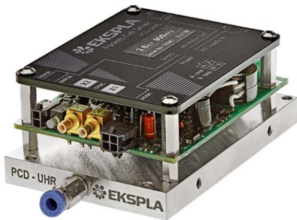
Fig. 17. OEM version of PCD-UHRS series driver with general purpose pad
