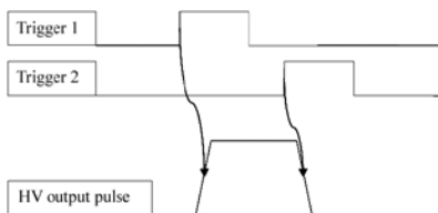
Fig. 3. Control timing charts for two-pulses controlled drivers
