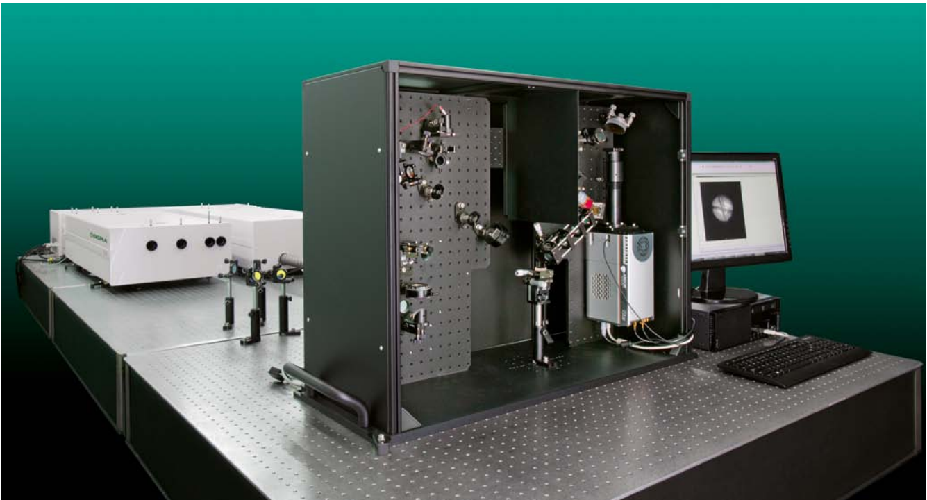
SFG microscope – provides spectral and spatial surface information with micrometers resolution.
