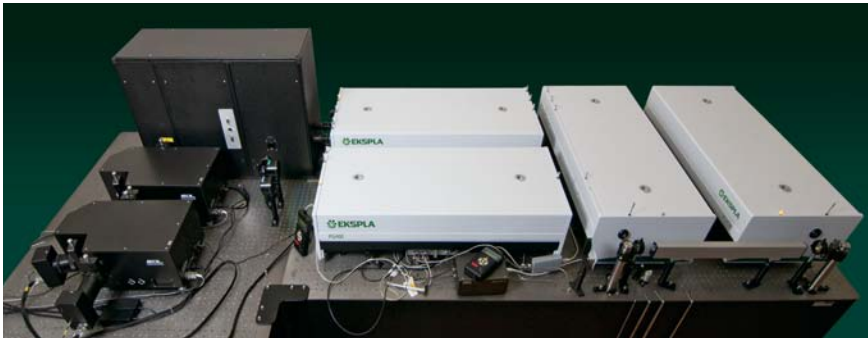
External view of Double resonance SFG spectrometer.
