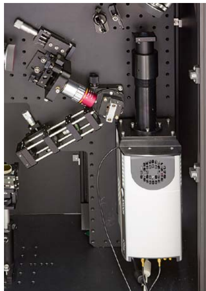
Detection part of SFG microscope.
